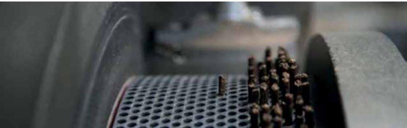
Organo-mineral granules being produced through extrusion (courtesy of Italtipollina)
