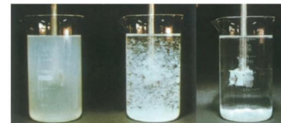
Separation into solid and liquid by flocculant (coagulation agent)
