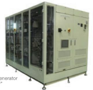
Electrolyzed sulfuric acid generator "GREEN SULFACEED KD™"
