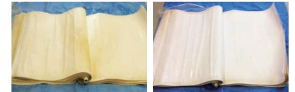
Slime peeling effect of RO membrane biofilm control agent (left: before washing, right: after washing)
